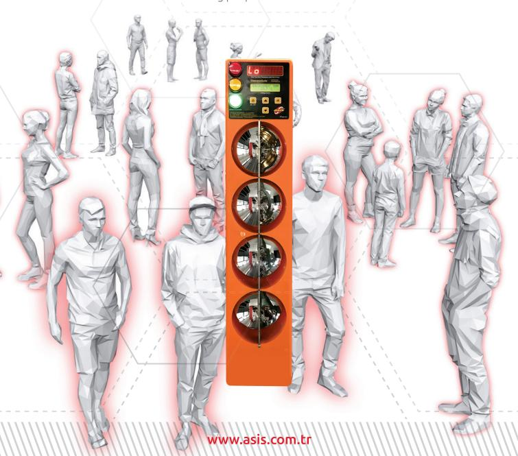
ThermoGate®, is 32-point precision IR thermometer designed for measuring the temperature of the human body and screening people who have fever. You just have to place it at the side of a door. When a person with body temperature over 38°C passes by, a red light and a beeper provide an alert.
